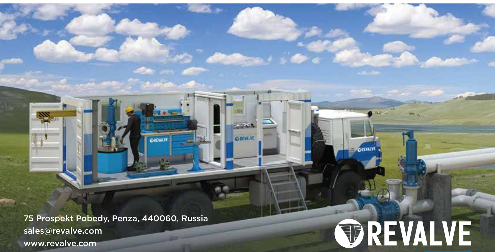
Vertical test bench for testing the wellhead and anti-blowout equipment
